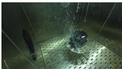
Length measurement sensor 48-hour rain-proof test
