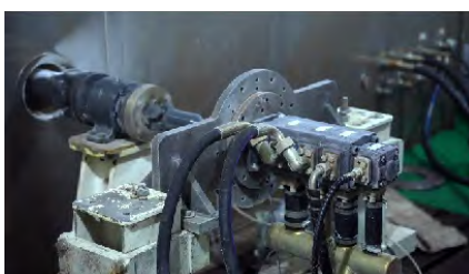
Hydraulic oil pump Low-temperature performance test under -40
