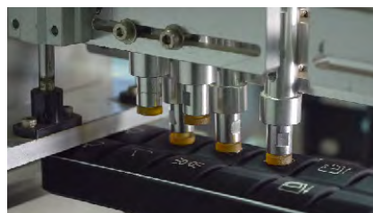
Panel buttons 1.2 million times reliability test
