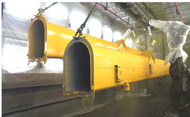
SPRAYING PROCESS OF ROBOTS
