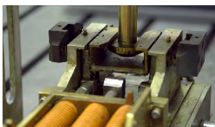
Telescoping mechanism Smoothness test
