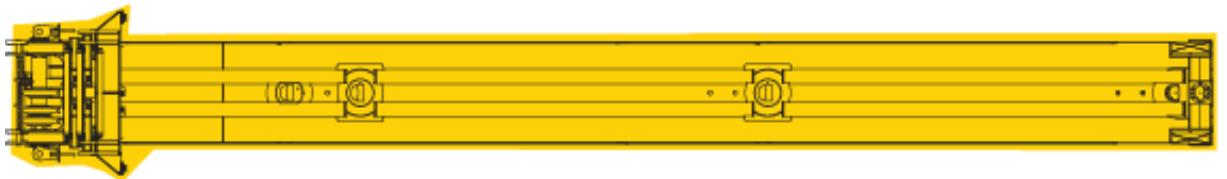
2<sup>nd</sup>- 4<sup>th</sup> boom sections; Weight: 26 t; Dimensions: 16500mm×1950mm×2450mm
