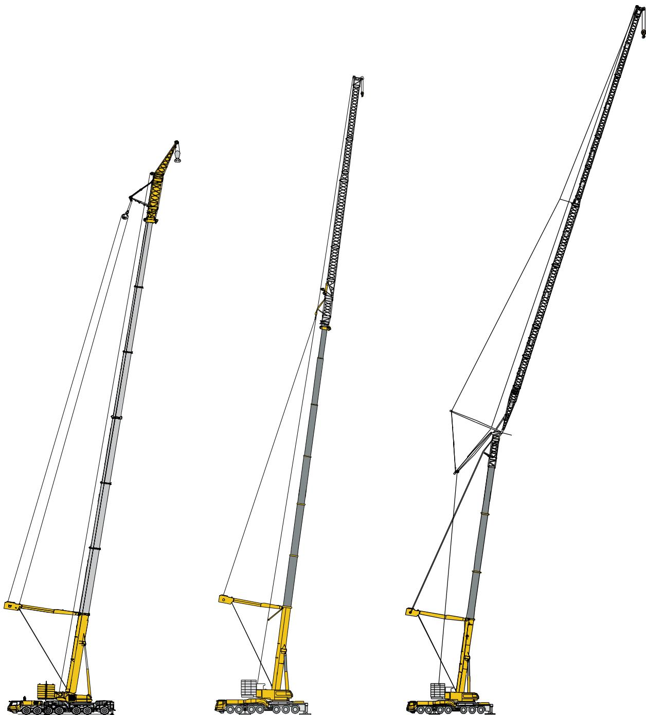
Super lifting device+ wind power jib
