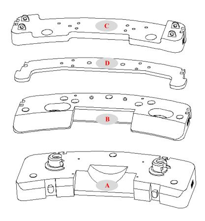
Note: Counterweight A is put in the middle of crane, and counterweight B, Cand D is fixed at the rear of crane
