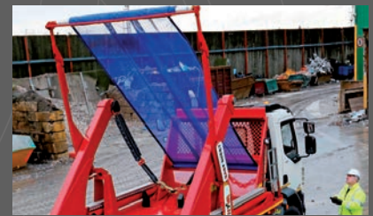
AUTO SHEETING SYSTEM
