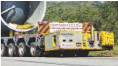
The rear-mounted PPU can be adjusted for uneven surfaces
