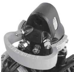
The hose guard is a metal bow to be attached onto the rotator. It is designed to protect the hoses of the rotator from damage i.e. from protruding branches
